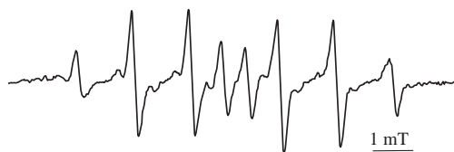
Fig. 3. ESR spectra of DPhPMPO-OH obtained in aqueous solution in the presence of HEG-Fe.
